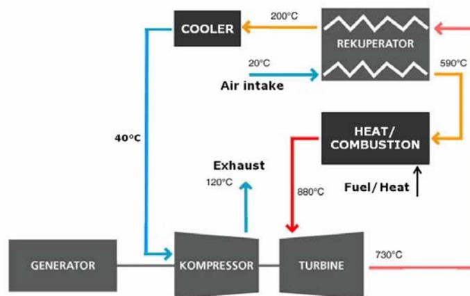
Figure 2 Scheme of an Aactor !GT inverted gas turbine
