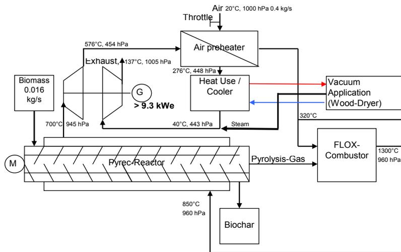
**Figure 4** Find the difference: Pyreg 500 with reactor iGT and additional steam intake from a vacuum application such as a vacuum dryer for furniture industry or food and drug processing.
