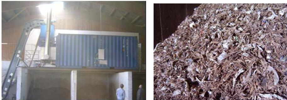
**Figure 1** First commercial Pyreg 500 plant near Lausanne (right) and typical biowaste which is not suitable for other use than Biochar: sand containing screen residues from a Kompogas-plant.
