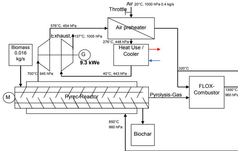
**Figure 3** Pyreg 500 Biowaste-to-Biochar plant with integrated iGT acting as exhaust fan and generating additional power (9 kWe). Please remark, that the 9 kWe is not the only gain of e-power – thus additional 4 kWe of power consumption of fans and blower can be saved.
