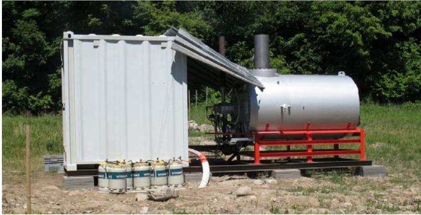
**Figure 6** 200 kWth pilot plant for the combustion of lean landfill gas. The connection for an Aactor !GT turbine is prepared. The LPG-gas (in the foreground) are only used to preheat the system. The nominal service is autotherm down to a 6% CH<sub>4</sub> / 94 % CO<sub>2</sub>.
